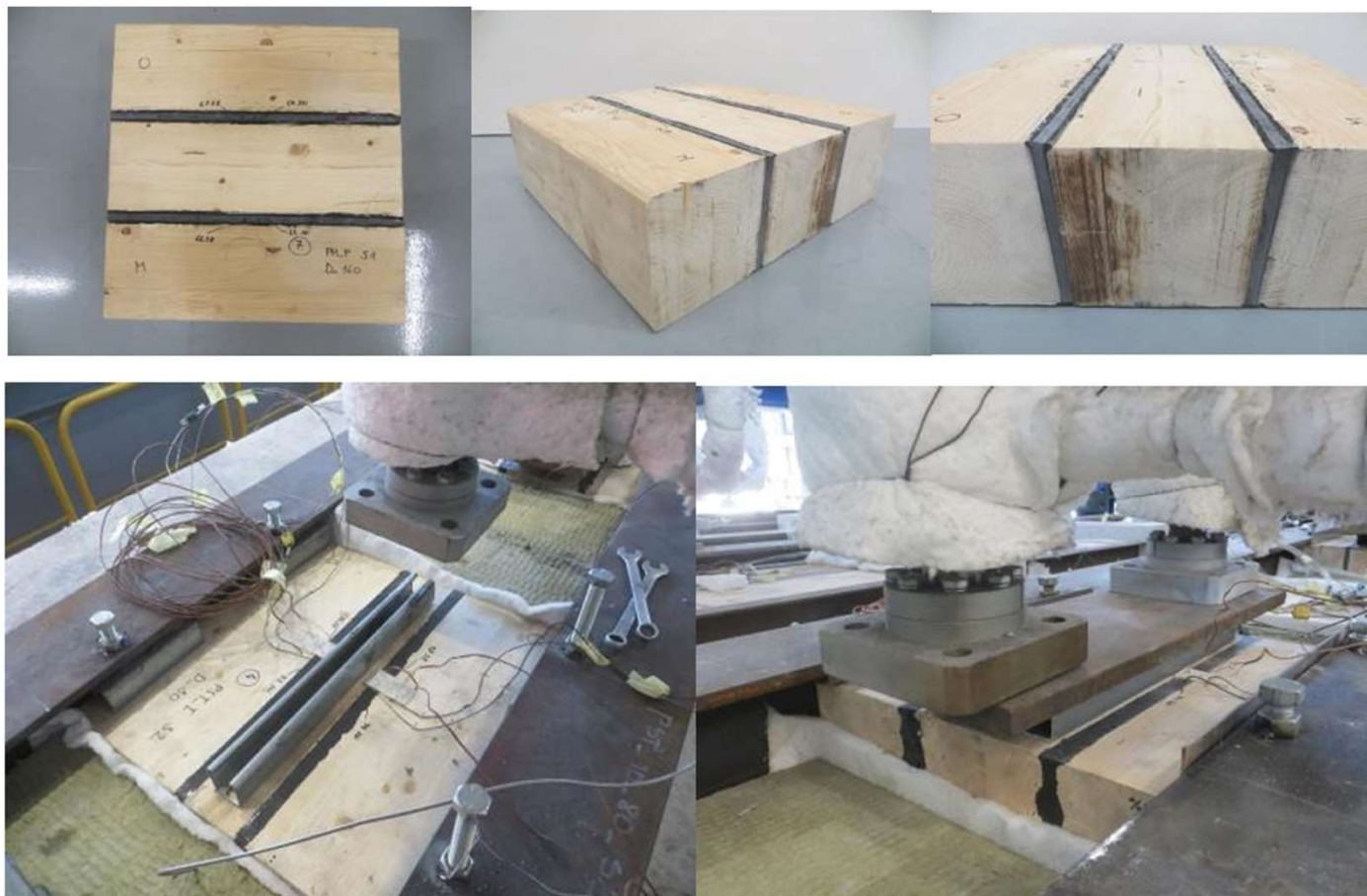
Photo A6.45: Hydraulic jack positioning for mechanical shear loading before the fire resistance test (photo archive, left: 049506d-222, right: 049506d-228)
