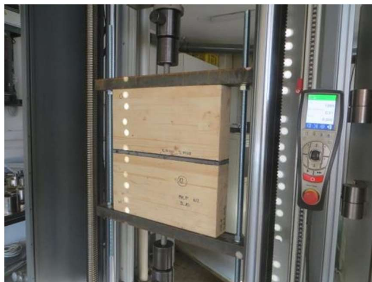
Photo A6.22: Mechanical loading of specimen no. 12 in tension (photo archive 049506d-069)
