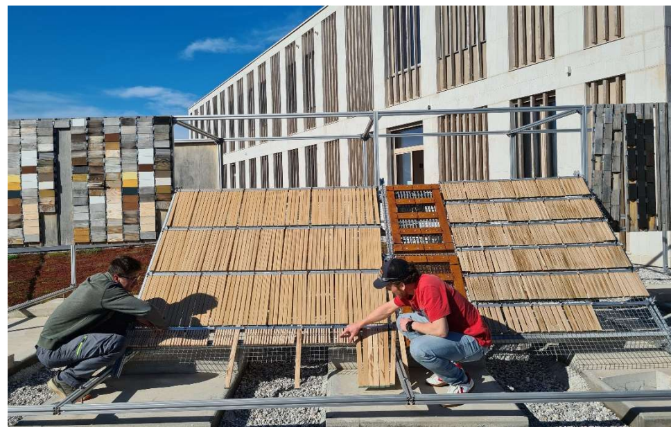
Natural weathering test site – Slovenia/Izola
