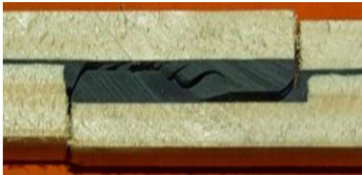
Shear failure mode
