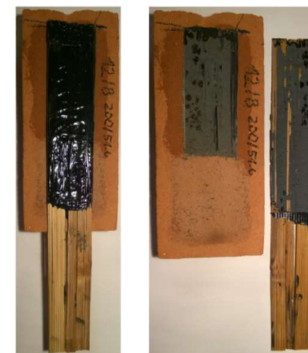
Single lap shear test (bamboo fibers vs. carbon fibers)
